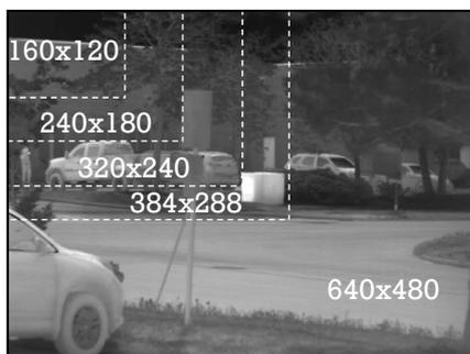
Relative pixel number comparison for thermal detectors with different resolution. The thermal image on the right was taken through a high-resolution FPA (640x480) and a front lens with low f-number ( $f/1.0$ )
