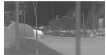
*Sensitivity of 50mK means that the detector is able to distinguish two objects with temperatures of 11.25 and 11.75 degrees respectively.*
