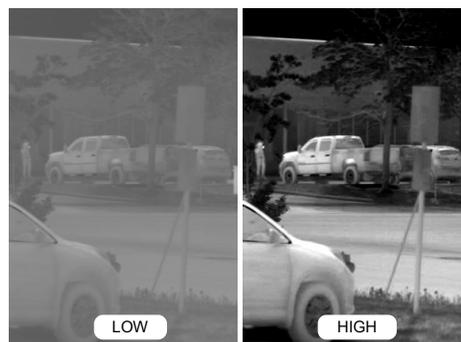
Now imagine, for example, an environment with uniform ambient temperature: a forest early in the morning. Operating in these conditions, you would need to **increase FPA sensitivity** to better distinguish temperature difference of surrounding objects. On the other hand, in the environment with temperature-contrasting objects (very hot and very cold), one may need to **reduce FPA sensitivity** to level out displayed image and achieve the best image perception.
